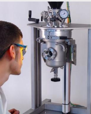
Visual control of reaction with glass reactor or sight glass
